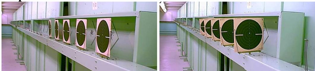
Target turning units for five (picture) and single targets are available. Target turning units can be chained and operated with a single controller.
